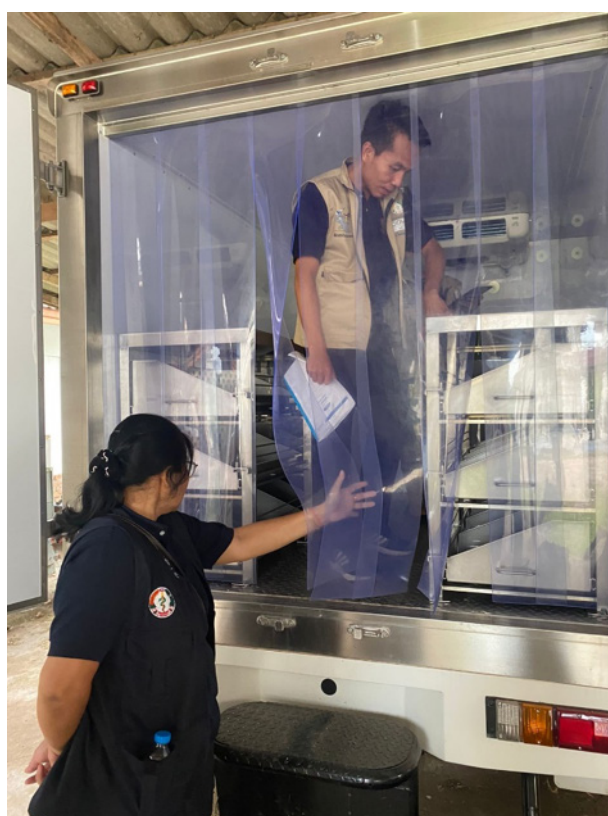
Figure 21: Team inspecting the racks inside the refrigerated van for transportation of vaccine
