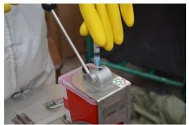
Figure 35. Mutilating syringes using manual needle cutter
