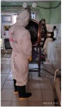
Figure 31. Loading the bio-hazard drum in pre-vacuum autoclave for disinfection
