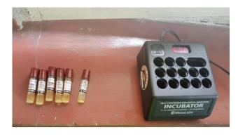
Figure 32. Incubating SCBI for checking growth of high temperature resistant bacterial spores
