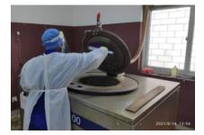
Figure 24. Closing the door of the microwave for disposal
