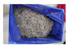
Figure 25. End product after disinfecting in the microwave with shredder
