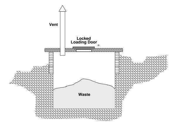
Figure E2. Cross - Sectional view of secured disposal pit for PHC organic waste
