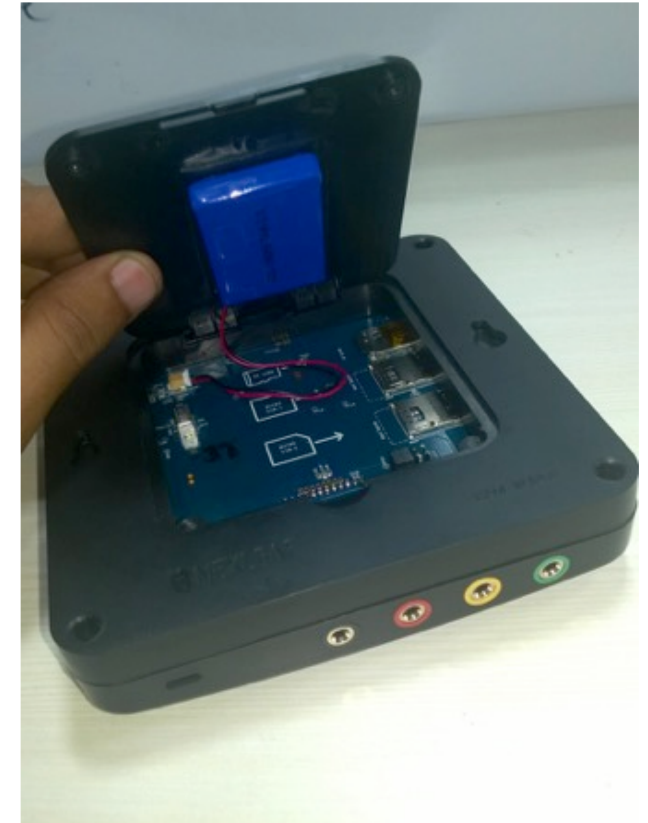
The battery is now connected to the plug and the back cover.
