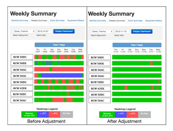
**Figure B:** Screenshot of ColdTrace dashboard weekly summary showing performance of 8 fridges before and after thermostat adjustment.
