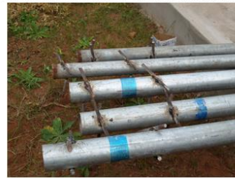
Nominal Galvanized Steel Pole and Aluminum Cap
