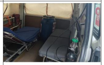
**Photo E.5.6.** Installation of a bio hazard container inside an ambulance.
