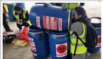
**Photo E.3.5**. Installing testing kits, including biological spores and chemical integrators ,inside bio hazard containers.
