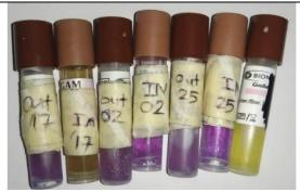
**Photo E.11.5.** Result of waste disinfection shown in spores after autoclaving the waste
