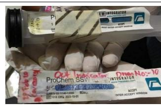
**Photo E.12.5.** Result of waste disinfection shown in spores after autoclaving the waste
