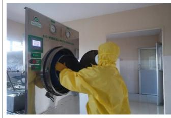
**Photo E.13.1.** Loading a bio hazard container into a pre vacuum autoclave
