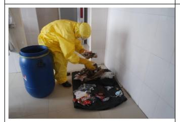
**Photo E.13.3.** Waste segregation after autoclaving the waste
