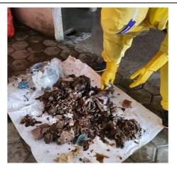
**Photo E.12.3.** Waste segregation after autoclaving the waste
