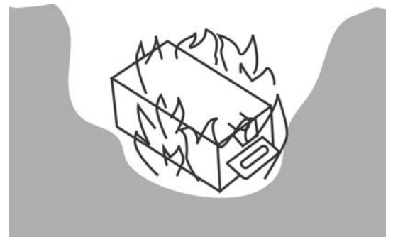
Figure 3.12 Open burning in a pit
