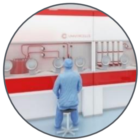
Polio vaccine production Isolator-based micro-facility
