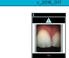
The device has detected movements during the analysis. Please redo the acquisition without moving during one second (time of the acquisition). See point «6.1. Introducing the right way to use the Rayplicker<sup>™</sup> device», page 20.
