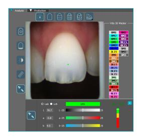
Calculate to the nearest pixel the color difference "Delta E or  $\Delta$ E" between the actual shade of the tooth and the closest shade according to the selected reference shade guide.
