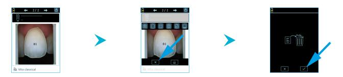
The first way to delete one (or more) acquisition(s) saved on the Rayplicker $^{\text{\tiny{M}}}$  device is to make it directly from the file explorer:
