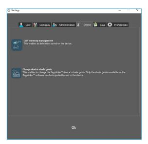
To delete one (or more) acquisition saved on the Rayplicker<sup>™</sup> device, this can be done using Rayplicker<sup>™</sup> software.
