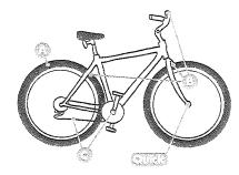
A is for air: Inflate tires to pressure rating on the sidewall of tire and check for damage.
