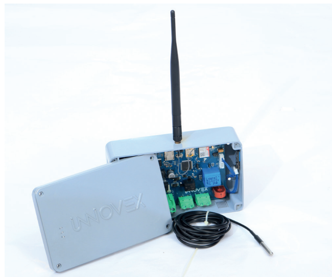
Image: Innovex's 'Remot' IoT hardware with front cover removed
