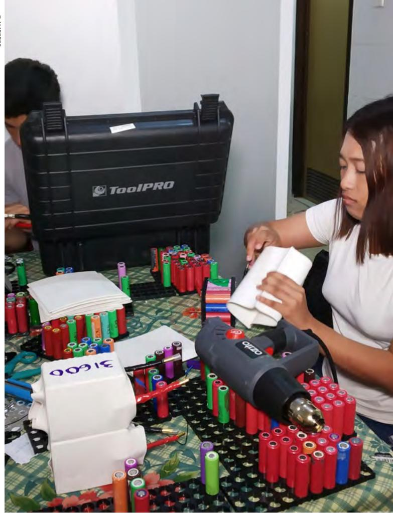
Heat shrinking as part of battery upcycling from e-waste (Myanmar, 2020)
