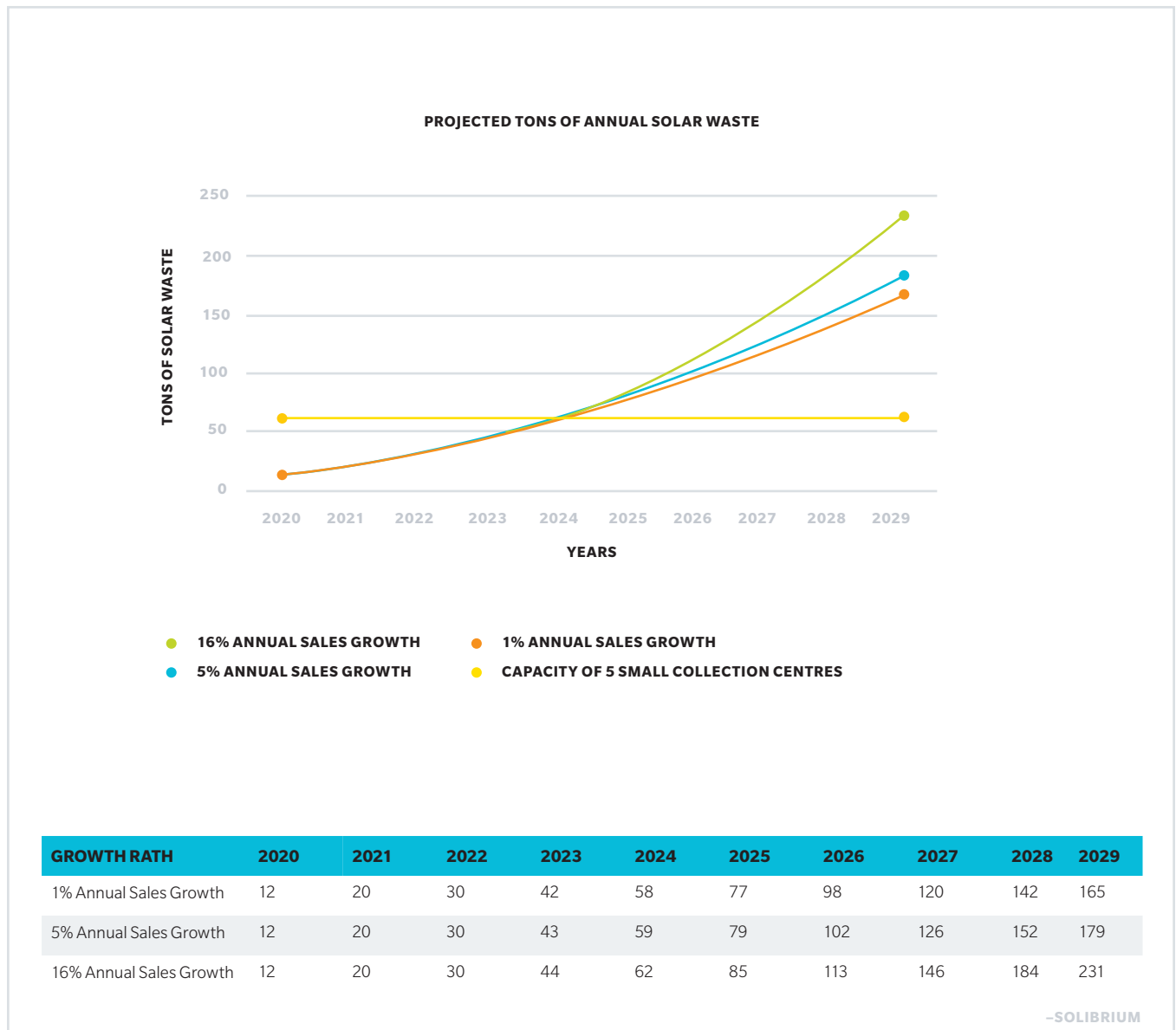
Figure 10: Projected yearly tonnes of solar waste in Kakamega County, Kenya, with three annual growth scenarios from Solibrium.
