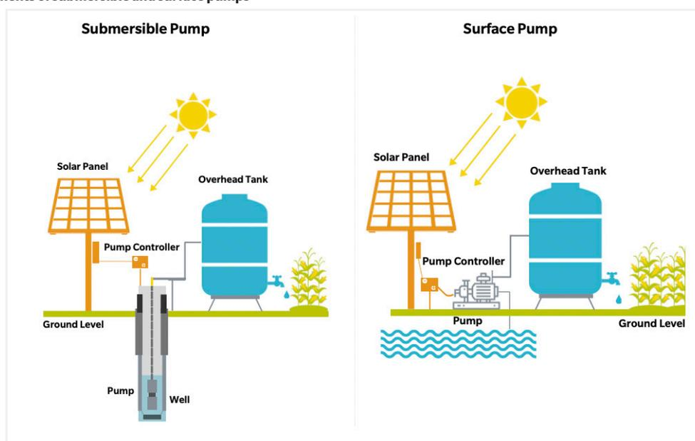
Although different pump types have varying components, the factors affecting the performance of a SWP are:
