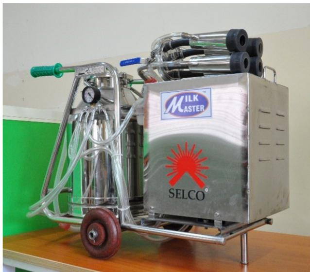
This machine can also be operated manually through a hand lever during power failure. It consumes very low power and can run on an inverter of 800 VA capacity.
