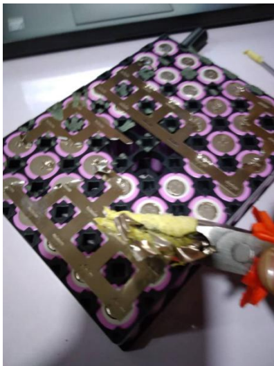
Figure 10: Top (left, 3 strip blocks) and bottom side(right, 2 strip blocks) connecting strips
