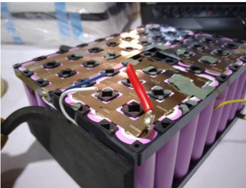
Figure 7: Removing the insulation and shock absorber foam
