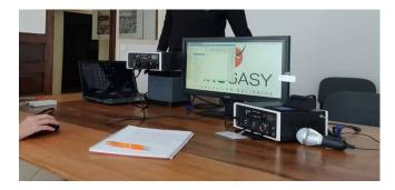
The remote monitoring feature can also lock and unlock the computer remotely. This is important for security reasons, but also enables a more affordable PAYGo option, as Jirogasy can enable the computer when a customer makes a payment.
