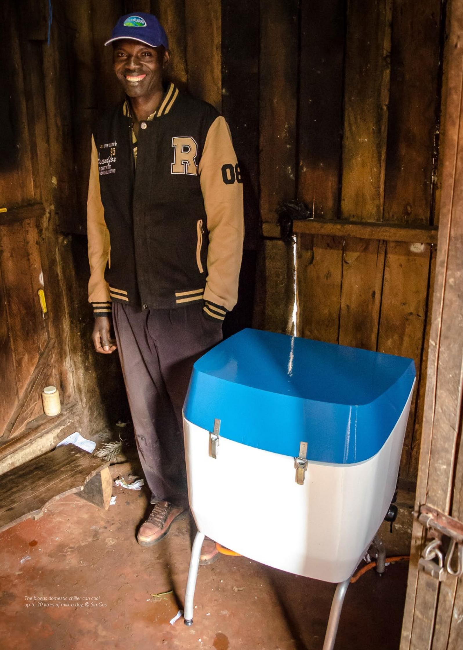
The biogas domestic chiller can cool up to 20 litres of milk a day. © SimGas
