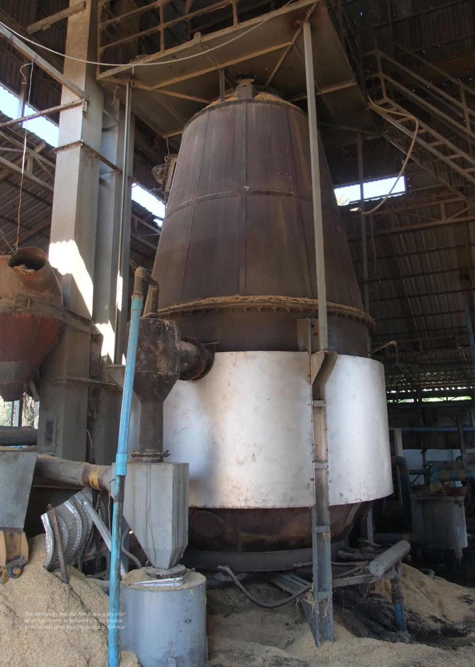
The technology provider Ankur sells a dry char discharge system to separate the dry biochar from tar and other liquid by-products. ©Ankur
