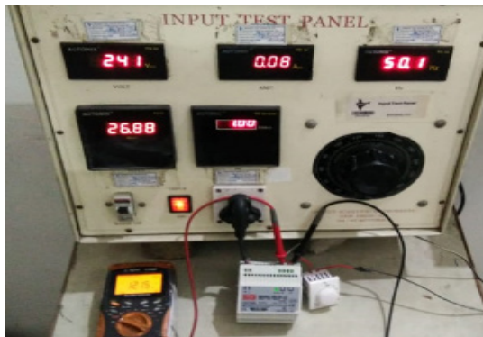
Figure 28 – Testing of DC fans with rectifiers
