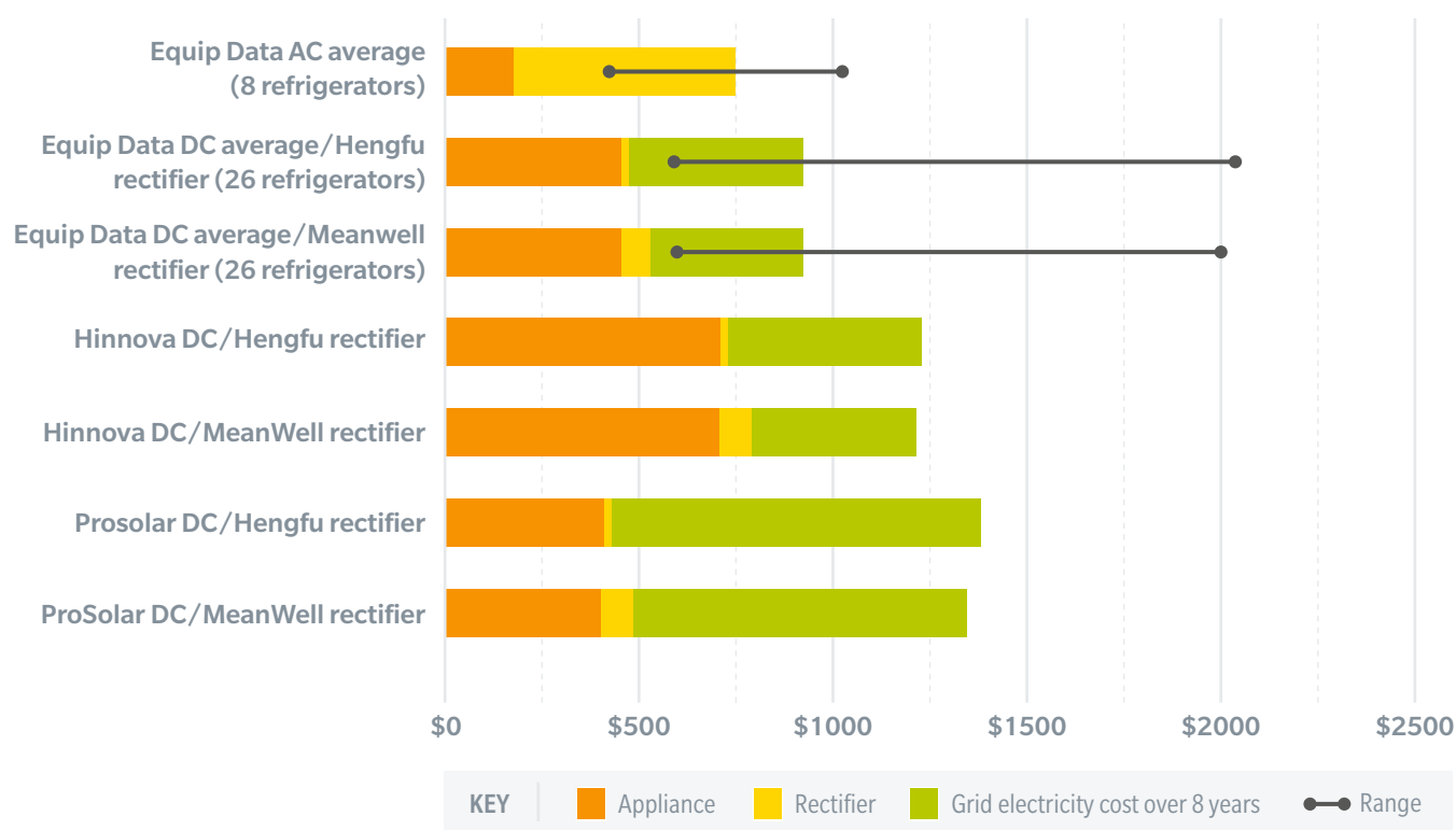
Figure 21 – Simple lifecycle cost of the tested DC refrigerators with rectifiers running on an AC mini-grid, and comparison with average AC and DC models from Equip Data
