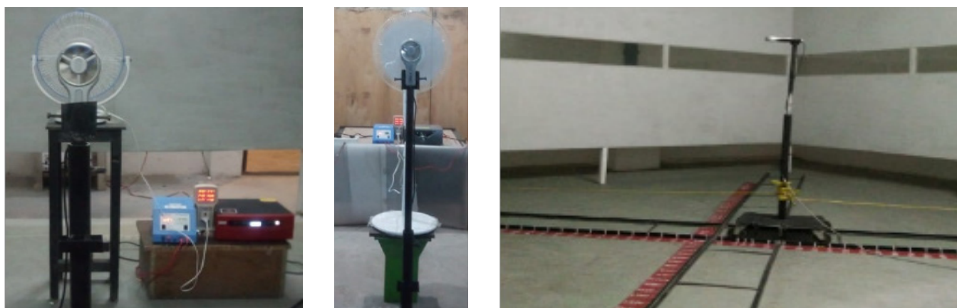
Figure 27 – Testing of the AC fans with inverters
