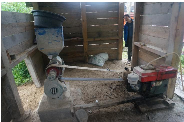
**Figure 10: Diesel powered milling machine**
