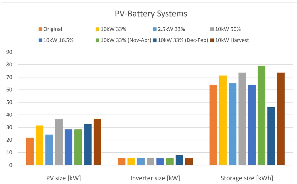
**Figure 21. Optimal generation sizing for PV-battery systems**
