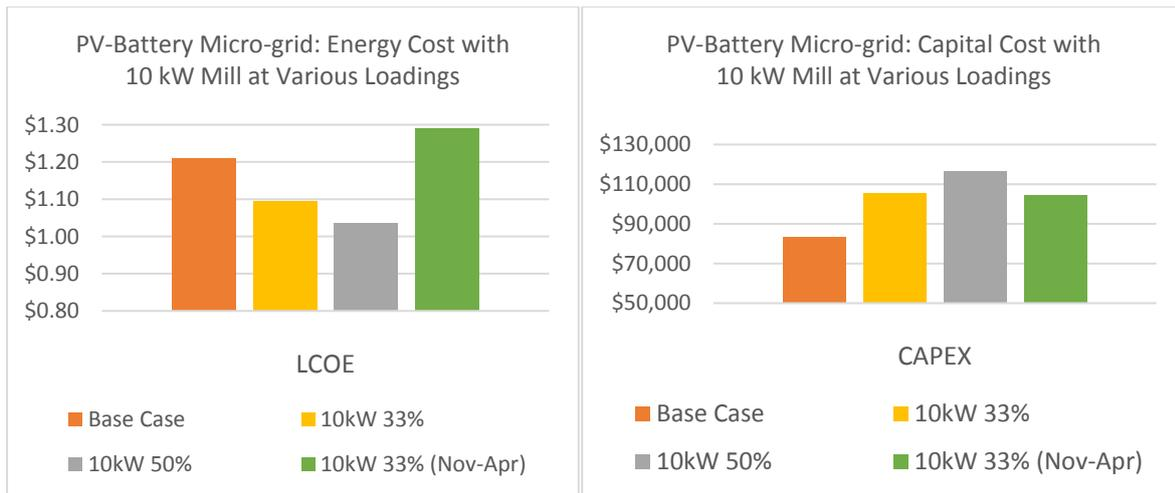
**Figure ES-2. Levelized cost of energy (left) and capital expenditures, or CAPEX (right) for photovoltaic-battery system with a maize mill in Tanzania**
