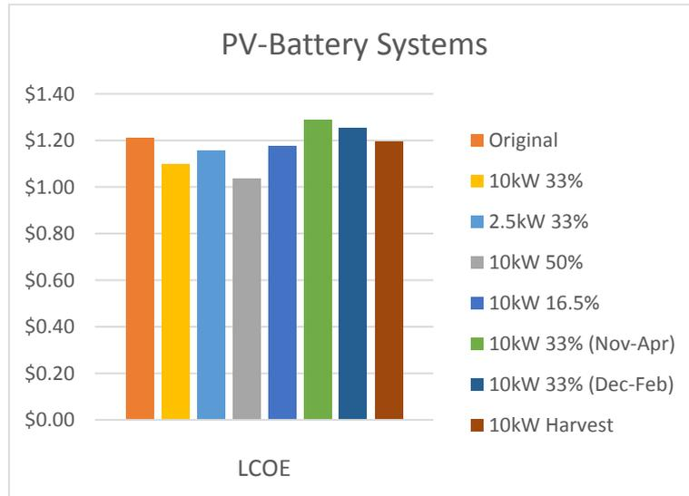
**Figure 19. LCOE of PV-battery systems (\$/kWh)**
