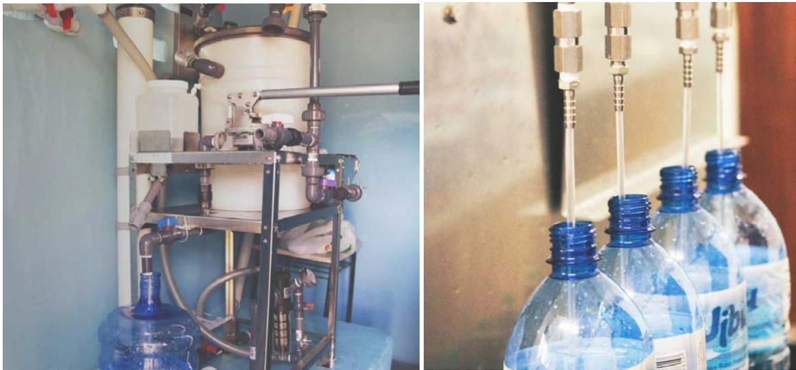
**Figure 13: Healing Waters treatment system and bottle filling**
