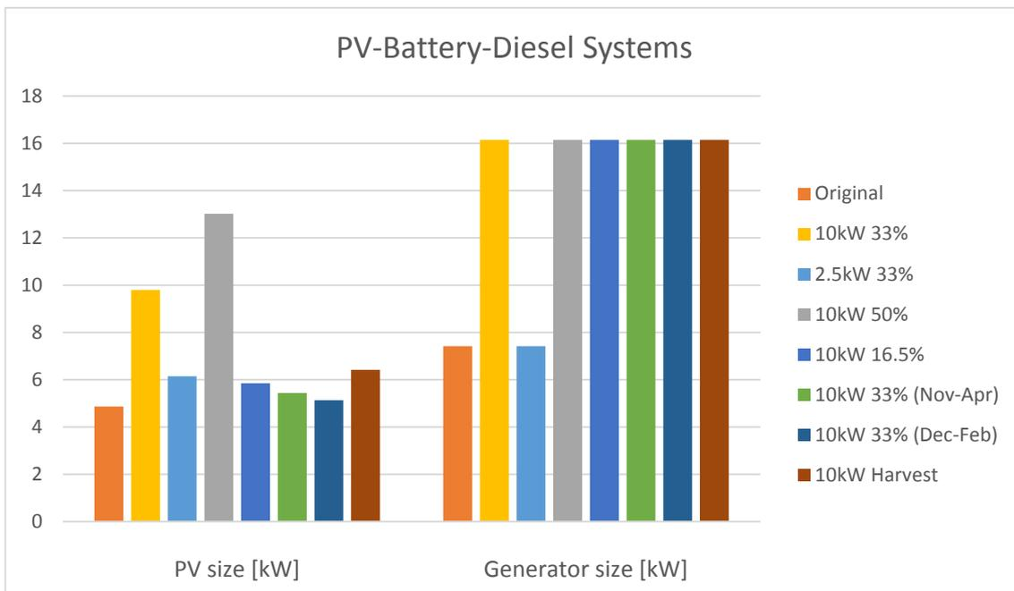
**Figure 18. PV and generator sizing for hybrid systems**
