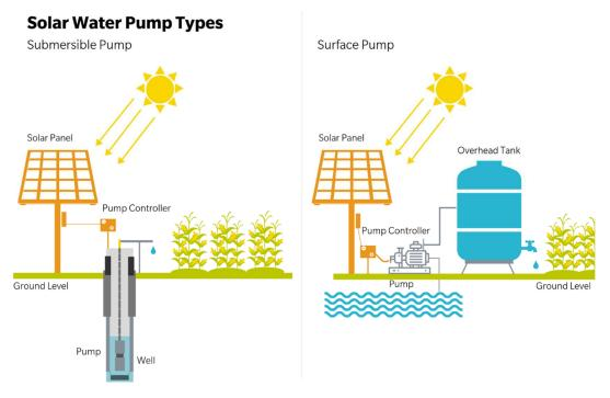
Figure 4: Representation of a submersible and surface pumps.<sup>10</sup>
