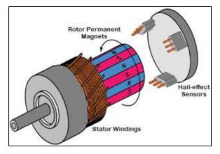
Figure 13: BLDC motor construction.65
