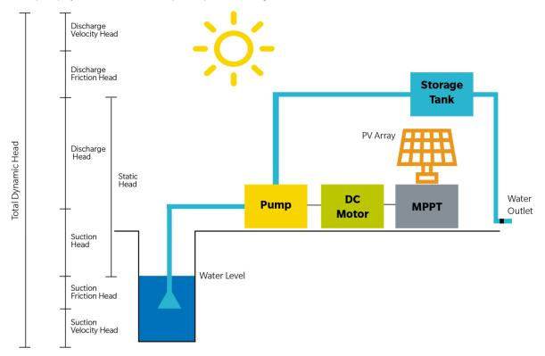
Figure 2: A schematic diagram of a PV water pump system with MPPT and DC motor.<sup>2</sup>
