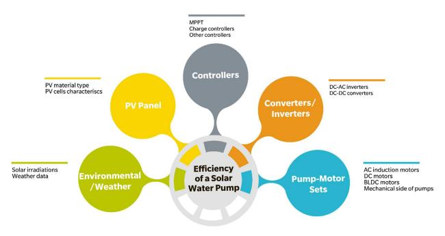
Figure 5: Key factors influencing the efficiency and performance of a solar water pump.
