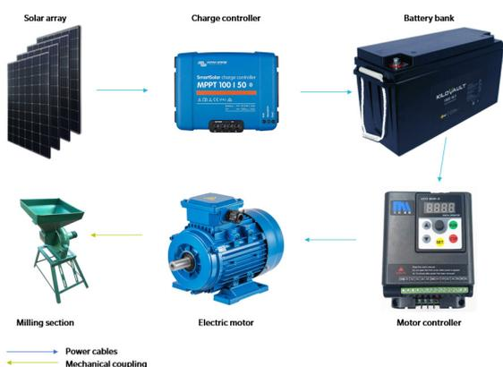
Figure 3: Layout of a direct-drive solar mill<sup>47</sup>
