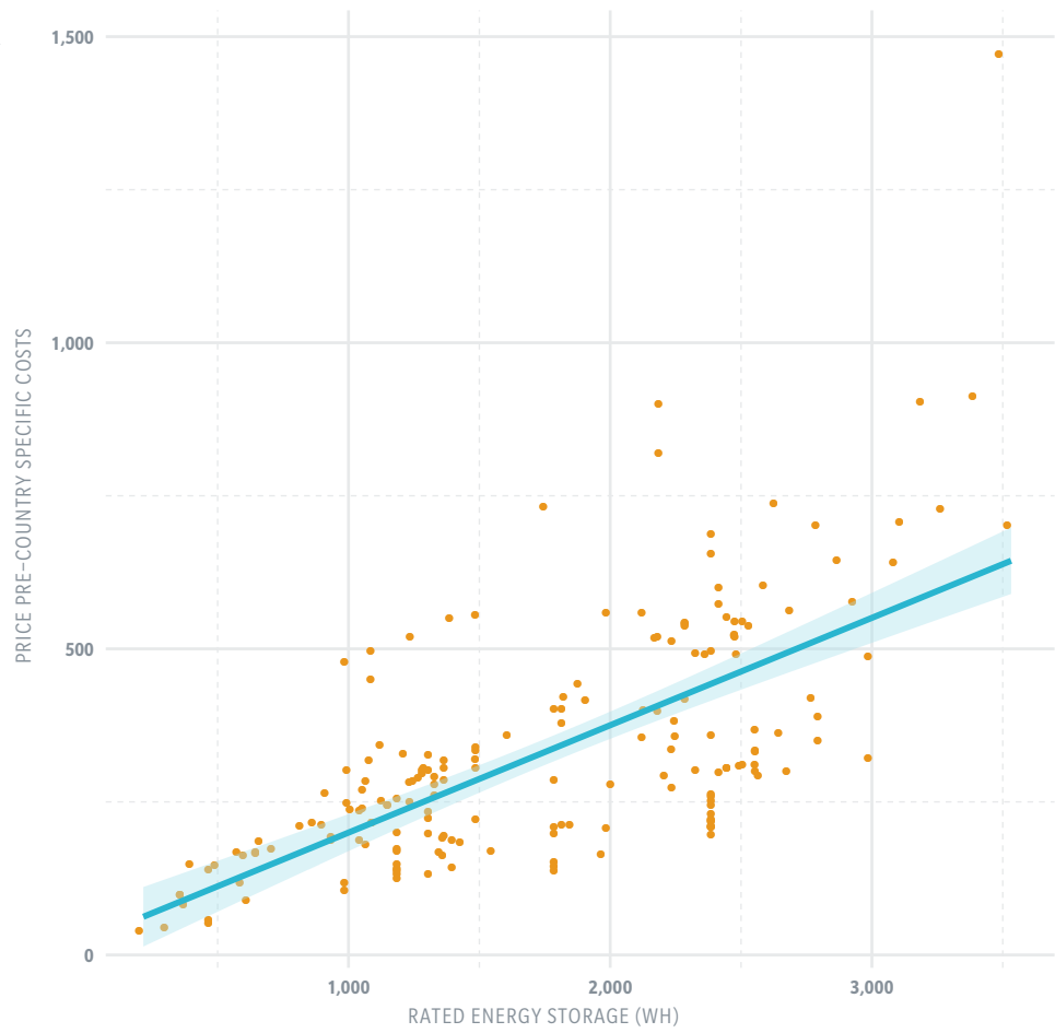
Figure A.3. Lead acid battery linear model.
