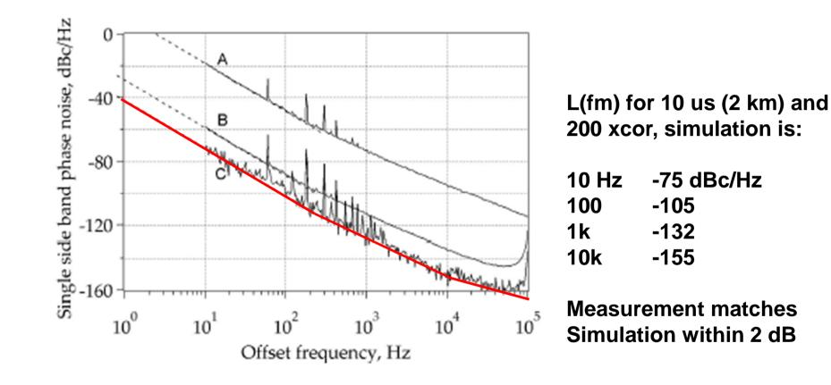
Note: Measurement is from an older prototype than actual measured data used in simulation and fiber link had a higher residual noise but matches Simulation on old data within 2 dB.
