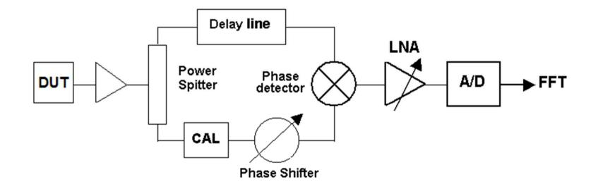
τ: Time Delay between the 2 paths, Delay-line length
