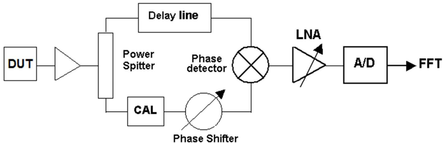
$\tau$ : Time Delay between the 2 paths, Delay-line length
