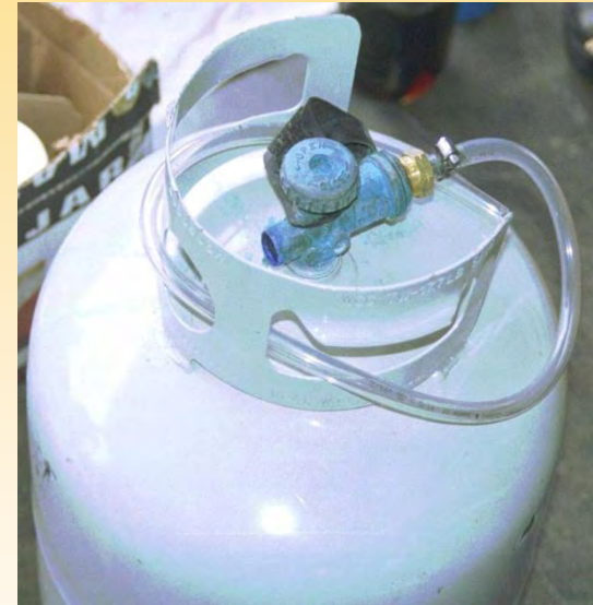
Propane tank used to store ammonia – note the blue tarnish on the valve fittings
