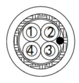
Cable Marking: RS PRO 4 Core×0.25mm<sup>2</sup> Screened Industrial Cable 250V
