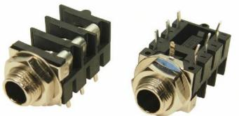
This 6.35mm Stereo jack socket has a metal nose and removable front earth washer. The body material is PBT UL V0 with an aluminium nose, and the contact material is brass / nickel plated.
