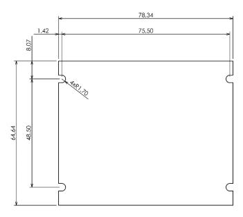
All dimensions are given within +/-0,5mm tolerance
