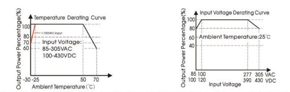
Note: 1. With an AC input between 85-100V/277-305VAC and a DC input between 100-120VDC/390-430VDC, the output power must be derated as per temperature derating curves;
