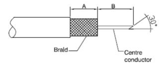
2) Twist the braid in a clockwise direction so that a minimum of 1,0mm dielectric is shown. Make sure to avoid loose or stray strands that could cause short circuits.
