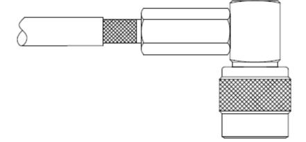
Firmly push the cable as far forward as possible and screw the connector hex back end onto the cable in a clockwise direction until it stops.
