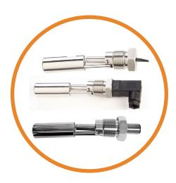
The SSF212 series are horizontally mounted switches that are fitted via a 1/2"NPT thread from the outside of the tank, so does not require access to the inside of the tank.
