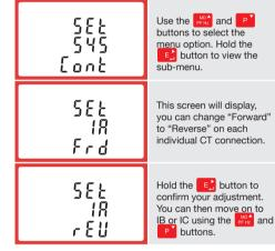
Hold the **W**<sup>A</sup> button for 3 seconds to exit the set up menu.
