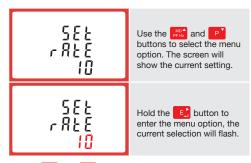
Use the wind and without to choose the desired pulse rate. To save the new setting, hold the c button for 3 seconds until the selection stops flashing
