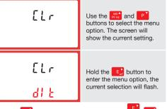
Hold the E button to confirm the setting and sets MA to return to the main set up menu.
