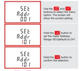
Use the Final and Final buttons to choose the necessary number, then press the Ei button to move along to the next number. To save the new setting, hold the Ei button for 3 seconds until the selection stops flashing
