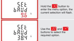
On completion of the entry procedure, hold the 🛃 button to confirm the setting.
