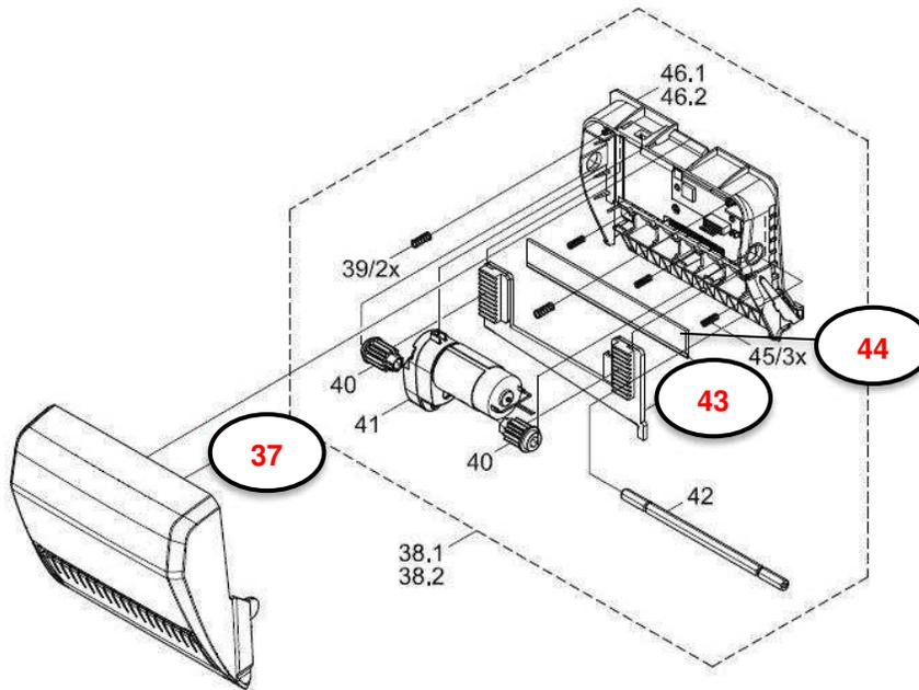
Figure 3 - T2212-PRINTER CUTTER/PERFORATOR
