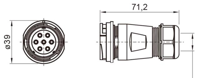
Cable outer diameter range: 13-16mm
