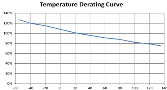
Calculation for ideal fuse selection =  $\frac{\text{Operating Current (A)}}{\text{Rating (\%}\times 0.75)}$
