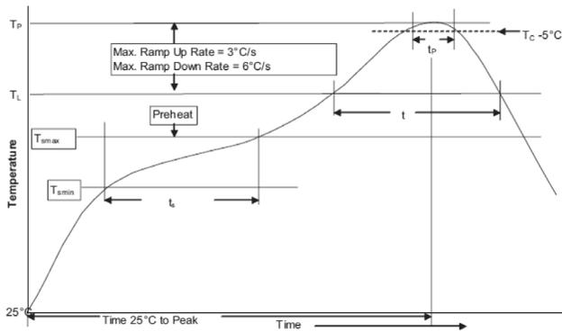
1. Infrared Reflow: Temperature: 260°C
