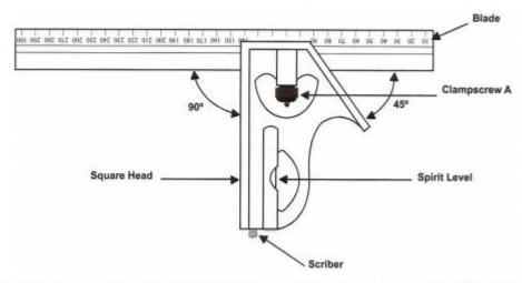
Note: Graduations are on both edges of the blade. Diagram shows only on one edge as it is intended for general information only
