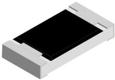
The resistors are constructed in a high grade ceramic body (aluminium oxide). Internal metal electrodes are added at each end and connected by a resistive paste that is applied to the top surface of the substrate. The composition of the paste is adjusted to give the approximate resistance required and the value is trimmed to within tolerance by laser cutting of this resistive layer.
