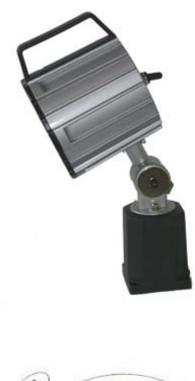
Lamp head made of die cast aluminium. Fitted with thumb switch. Fitted with: 1 halogen lamp 70 watt. Dimensions: Lamp body: 125Ø X 130 mm. Special articulation base. Enclosure type: IP 65 Class of protection: I Mains lead: 1.8m Supply Voltage: 110V / 230V
