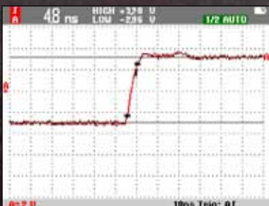
5GS/s sampling or 200 ps sample resolution provides the detail needed to inspect signal edge dV/dt or signs of destructive reflections.
