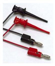
1 pair (red, black) of test leads with multi-stacking 4 mm banana plugs and mini-pincers Mini-pincers open to 2.3 mm 90 cm long PVC insulated leads 30 V rms or 60 V DC, 5 A One year warranty
