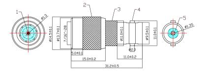
Item Designation Material Pin Cu 1 2 TNC Shell Cu 3 Body Cu 4 Zn **BNC Female Part** 5 Dielectric POM
