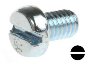
Cheese Head machine screws are designed for ease of assembly and this variety of machine screws with slotted drives are a popular driving method with this type of fastener. Machine screws can be used in pretapped holes or used with conforming nuts and washers in through holes.
