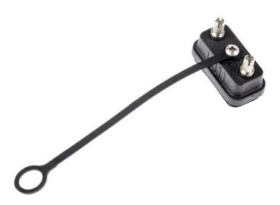
The RS Pro protective dust caps are used with a wide range of RS Pro D-sub plastic panel mount connectors. The IP67 rated black thermoplastic dust covers prevent water and dust ingress when panel mount D-sub connectors are not in use. Ideal for industrial applications and harsh environments.
