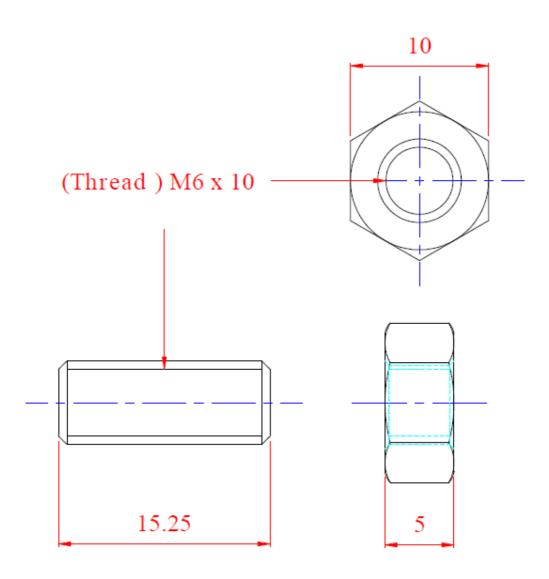
Material: Cold Rolled Steel
