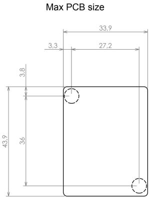
Dashed line shows outline of the mounting boss under PCB board Recommended mounting holes diameter ø3,5mm All dimensions are given within +/-0,5mm tolerance
