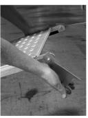
7.Place the Work Platform on the third rung down between the outer ladder bases. The wire hooks of the Work Platform should rest on the outer rung that faces inward.
