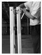
4. Place one of the lock tabs into the hole of the second outer section. Repeat on the other side.
