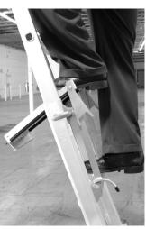
2. Push the Work Platform forward as shown above. Climb the ladder up to the rung above the platform.
