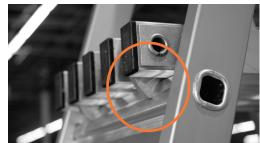
The Telescoping Plank has two safety hooks on each end that keep the Plank from sliding off the trestles when placed correctly.
