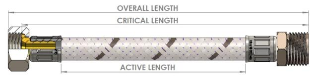
Critical length is the distance between hose mating faces. This must be 10% greater than the actual distance between the two corresponding fixed mating parts to avoid tensile stress whilst in service.
