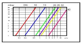
Schedule 2: Pressure loss for type of end connection based in internal diameter (DN) Formula:  $P2 = P3 \times R$
