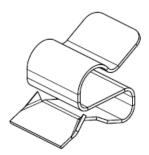
SINGLE CABLE GIRDER CLIP TO SUIT Ø8-9 CABLE AND 2-4 THICK FLANGE. ZINC PHOSPHATE SILVER COLOURED SACRIFICIAL COATING (Z600+) WITH WATERPROOF TOPCOAT. COATING IS CHROMIUM FREE.
